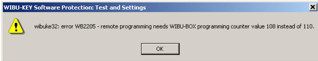
Please record the message on the error dialogue. Doing a *Print Screen* and saving the *bmp* file is the best way to record details of the error.
